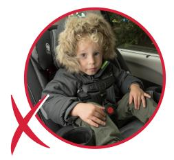
A bulky coat will make the seat harness fit incorrectly, which can cause injury or ejection in a car crash.
